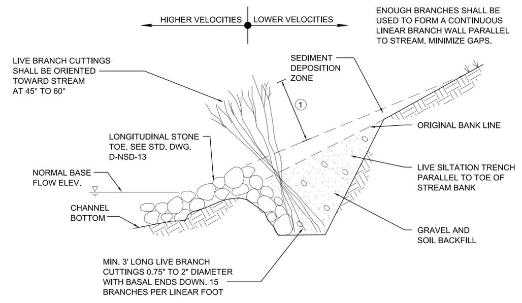
**SECTION VIEW - LIVE SILTATION WITH STONE TOE**
